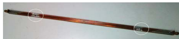
Fig. 4. Photo of the transmission line with two controllable loads
