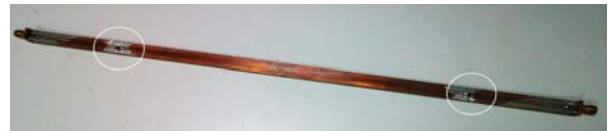
Fig. 4. Photo of the transmission line with two controllable loads
