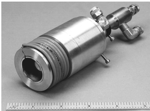
Fig. 1. Vacuum arc plasma guns. Upper: Disassembled simple uncooled version. Lower: This version includes water cooling and a small magnetic field to guide the ejected plasma stream
