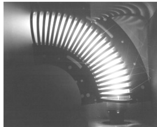
Fig. 2. Upper: Set-up for plasma deposition using a vacuum arc plasma gun with associated macroparticle filter. Lower: Photograph of plasma stream guided by a 90°-bent filter
